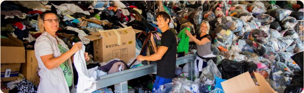
Textile sorting: collected textiles are sorted by hand according to their condition and their potential for reuse, redesign or recycling.
